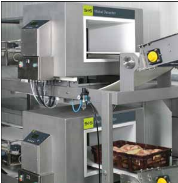
GLS metal detectors installed in two production lines to analyse poultry.
