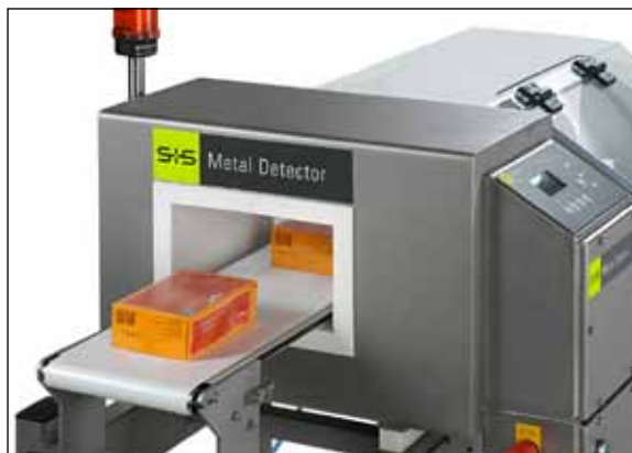
GLS metal detector: outgoing goods inspection for cookies.
