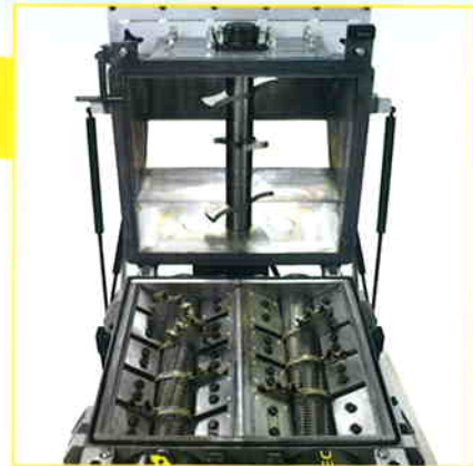
Open chamber and patented MASHER system
